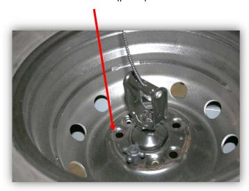
6. The spare wheel can be wound up by operating the winch with the crank. Wind the spare wheel all the way up until it locks automatically.
